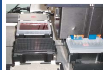
Figure 11. Multiple low volume dispense and wash cycles with disposable tips on the EP3. The dispense parameters for the EP3 were optimized for 0.5µl dispense of Artel's MVS Alternate Solution at 75% DMSO. Tips were loaded new and used to transfer 0.5µl of the Alternate Solution to the destination plate. A mix step was performed in the Alternate Solution prior to an aspiration of 0.1µl. After the transfer, a mix step was performed in the destination plate. The tips were then washed in a series of two water baths prior to the next transfer sequence.
